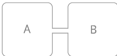
Figure 3: Isolated system made of two subsystems, to study the direction of flow of heat.
