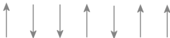
Figure 1 : System made of a collection of elementary magnetic moments. The elements are uncoupled among each other. The whole system is plunged in a magnetic field.
